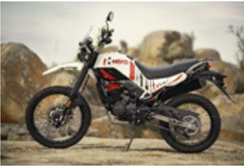
XPULSE 200 4V is an adventure motorcycle from Hero MotoCorp built for the thrill. It has a refined 200cc engine, and off-road-friendly components make it versatile and robust. It has a Rally Edition that comes with a factory-fitted Rally Kit, featuring a taller and fully adjustable front suspension and a fully adjustable 10-step rear suspension. The Rally Edition features the same colour combination as the Hero MotoSports Team Rally.
