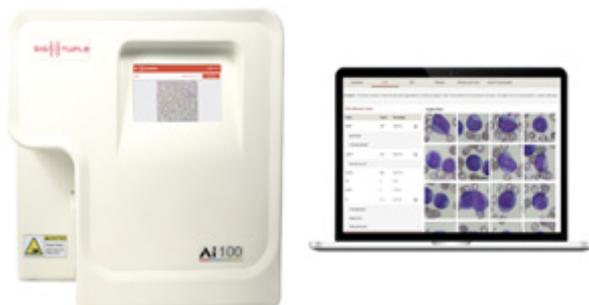
AI100 is an in-vitro diagnostic device designed to automate manual microscopy in a diagnostic laboratory. It uses robotics and AI to digitize any biological sample on a glass slide to enable AI aided remote review. Shonit is an AI application to analyze blood cell morphology, identifies and pre-classifies WBCs, RBCs and platelets in a peripheral blood smear. AI100 with Shonit gives an accurate 7 parts WBC differentials, NRBC, platelets and RBC morphology. AI100 with Shonit is currently an FDA
